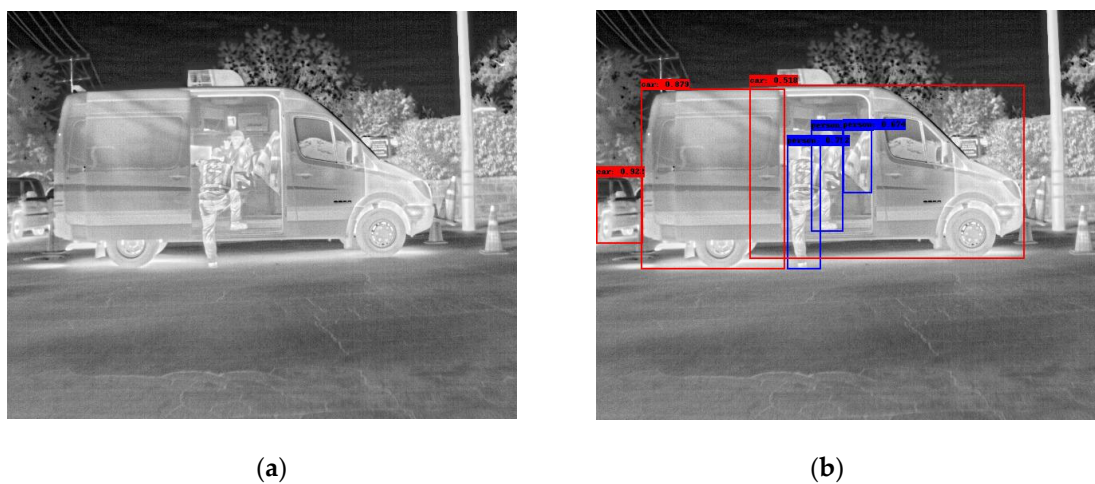
Figure 6. Detection example containing errors from the FLIR-ADAS dataset using YOLOv8. (a) The original image from the dataset; (b) the detected objects being annotated as overlaid bounding boxes. The car (van) is detected as two distinct instances.
